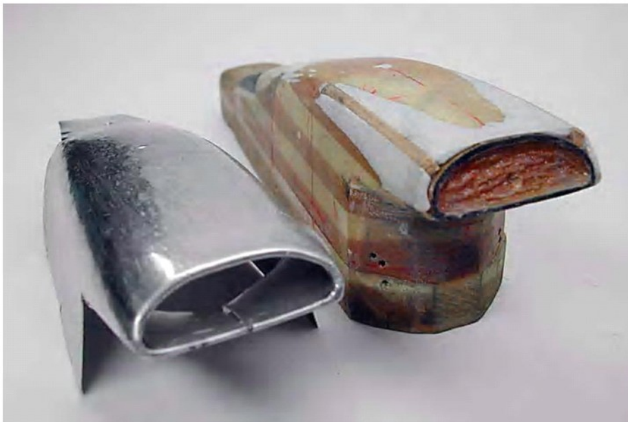
The form for the air intake and the final part. As is often the case in machining and model making, fixtures, moulds, formers and jigs to make the final parts can take a long time to make and are never seen by the public viewing the finished model. (Y. Park photo)
