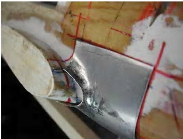
Each panel is hand formed over a wooden shape. The metal is annealed to the proper softness and then pounded and bent into shape. The plane is made up of many individual panels, and the fits between panels are just about perfect.. (Y. Park photo)
